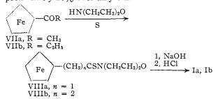
No attempt was made to isolate  $\beta$ -ferrocenylpropionothiomorpholide (VIIIb), but the yield of  $\beta$ -ferrocenylpropionic acid from hydrolysis of the crude reaction mixture was only 4%, reflecting the usually lower yields of product obtained from higher alkyl aryl ketones compared to those from methyl aryl ketones.<sup>12</sup>
